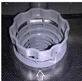
Poorly secured filter
